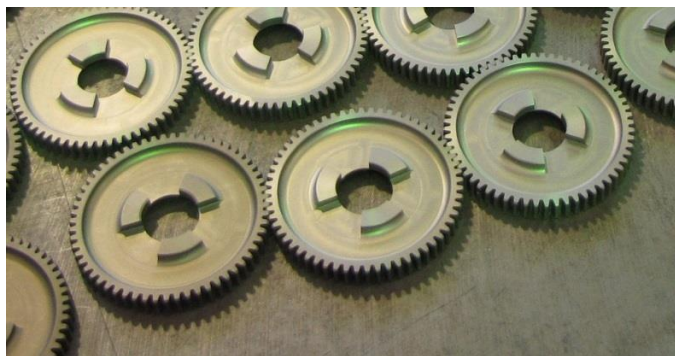
Automotive Gears made of AI-WQ68
